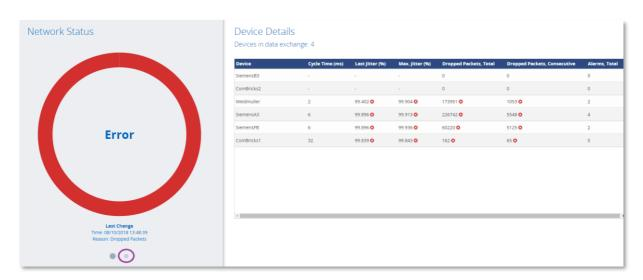
In case of errors, the large circle turns red as shown in the image. The right pane is a list of PROFINET statistics and errors per device.
