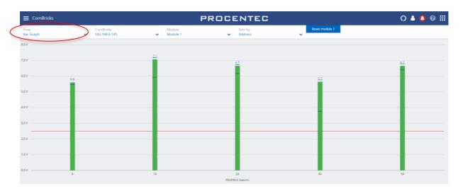
The 'Reset module x' button can be used to clear all Bar Graph data from that module. Resetting the Bar Graph in Osiris will also reset it in the ComBricks.
