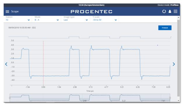
Figure 30 - Normal oscilloscope image of device 10
