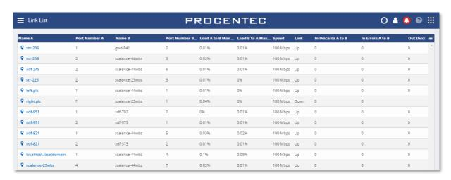
The table is adjustable, by clicking on the small menu button on the right. It is also possible to drag the colums wider or narrower (in the title bar of the table), so that the screen can display more information.
