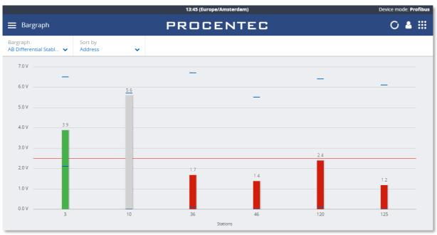
Figure 32 - Inactive and low bars
