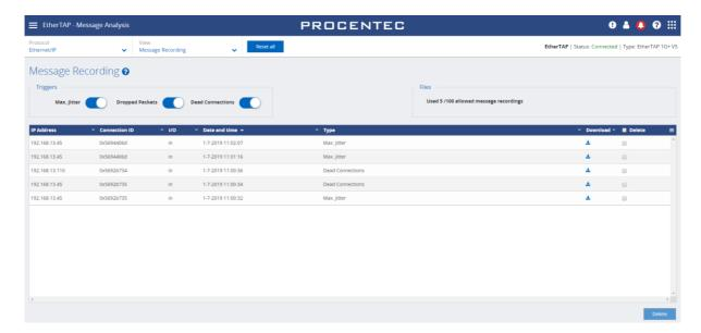
In this overview you can see the IP address of the involved device, the Connection ID, the I/O type of the connection, a recorded date and time, the event that triggered the recording, the file name, and a button to download or delete the recorded file.
