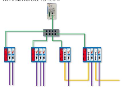
Figure 22 - One Atlas monitoring four different ComBricks
