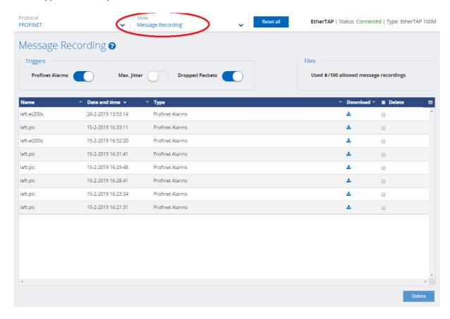
In this overview you can see the filename and a recorded date and time, the event that triggered the recording, and a button to download or delete the recorded file.
