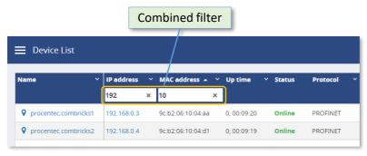
Figure 21 - Combined IP and MAC address filter
