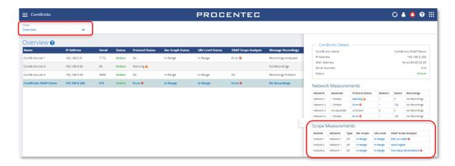
The Scope Measurements in the Details panel indicate some problems in Network 1, module 1, 3 and 4. In module 4 for example, the analysis is 'Too many terminations'. Clicking this line opens the SNAP analysis:
