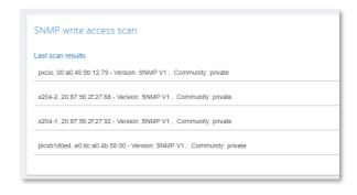
be possible and therefore a potential attack vector for the network. The devices in the resulting list should be changed, so that access via the mentioned community strings is no longer possible.
