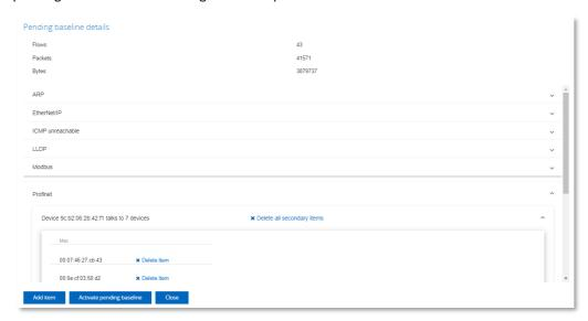
It shows all the connections, used protocols and statistics that have been observed during the baseline scan. The protocols can be expanded to view the MAC addresses that are communicating. In this window you can also add and remove items, to make sure that only the allowed devices and protocols are in the baseline scan. Adding an item requires the input of a protocol, a source, a destination MAC address and (if applicable) a source and destination IP address.
