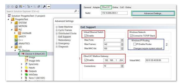
The IP address of the Mailbox Gateway/Diagnosis Interface in TwinCAT belongs to the subnet of the EtherCAT master interface, not to any LAN ports of the controller PC. The IP address of the master itself is also the gateway address to its subnet.
