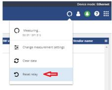
When the Relay has been triggered by an event, you can easily reset it in the Measurement menu (round spinning icon in the Icon bar), by clicking the 'Reset relay' menu item.
