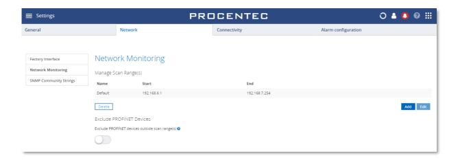
The network monitoring is performed on the Factory network interface, so it is important that the entire specified IP address ranges are reachable by Osiris through its Factory interface. To do this make sure your scan ranges falls within the subnet of the Factory interface.
