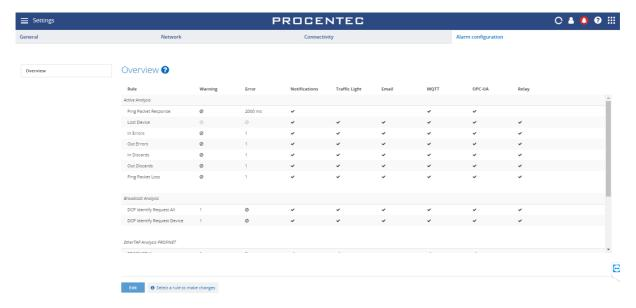
To change a line, select it and click the 'Edit' button in the bottom of the window. In the example below, the Ping Packet Loss alarms have all been disabled:
