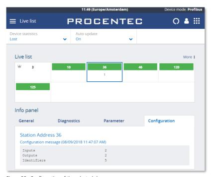
Figure 28 - Configuration of the selected slave.
