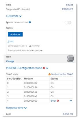
Figure 18 - PROFINET configuration: module 4 in error
