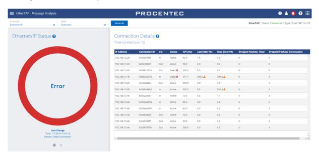
In case of errors, the large circle turns red as shown in the image. The right pane is a list of Ethernet/IP connections with statistics and errors.
