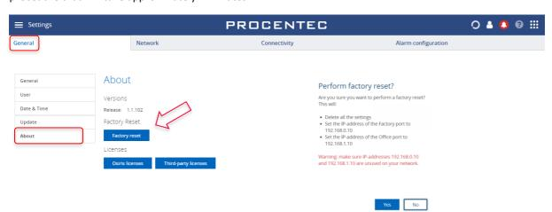
After the reset, it will reboot and be reachable on the default IP addresses again. You need to fill out the Setup Wizard before Osiris can continue normal operation again. Until that time, the yellow traffic light and the green RDY LED will blink on Atlas.
