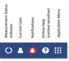
Figure 5 – Explanation of system buttons in web interface
