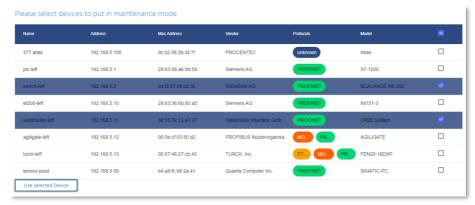
Figure 24 - Select the devices that need to be silenced during maintenance.
