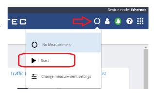
Figure 13 – Starting a measurement in web interface
