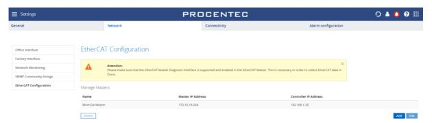
The Controller IP address must be within the Monitoring range of Osiris.
